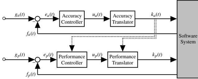
**Figure 1: Block diagram for controlling accuracy and performance.**
